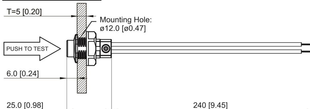
Dimension in millimetres [inches in brackets]
