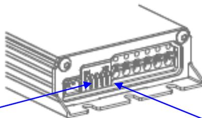
Dipswitch **1/2/3**: Setting LED working current in normal mode
